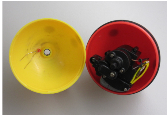
Fig. 2: The interior view of the “free” hemisphere (left-yellow) and the “fixed” hemisphere (right-red). The signal circuit components are also visible: the LED is mounted into the free hemisphere, and battery and leads are mounted to the motor assembly.
